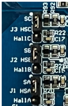
Figure 2-10 Actual Component Layout and J1, J2, and J3 Jumper Hardware Default
