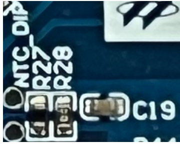
Figure 2-5 Actual Component Layout and NTC_DIP Position
