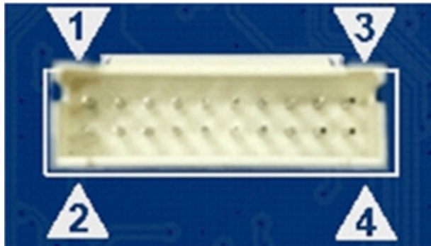
Figure 14. 20PIN (5PIN×4ICP) PHB Connector
